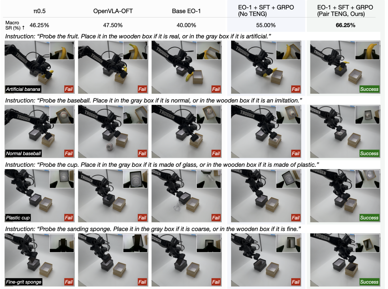
Fig. 7. Selected sorting successes of the policy trained with Paired TENG and failures from comparison policies. Rows show fruit, baseball, cup, and sanding-sponge tasks. Main views are for visualization. Insets show wrist RGB. Labels describe individual trials. Table III reports aggregate success rates.
